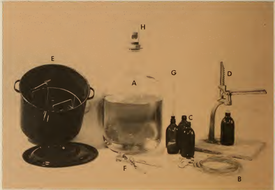
Figure 6. Small equipment and supplies. A, Five-gallon glass or plastic carboy. B, Four feet of 1/2-in. plastic or rubber tubing. C, Beer bottles for cider or juice. D, Capper. E, Canner with rack. F, Tongs to fit bottles. G, Thermometer reading to 230°F (110°C). H, Fermentation lock.
